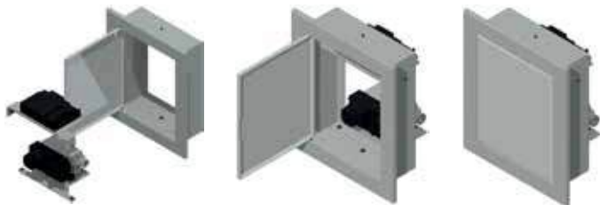
Figure 6. Mounting the gas controller with the receiver in the connection box
